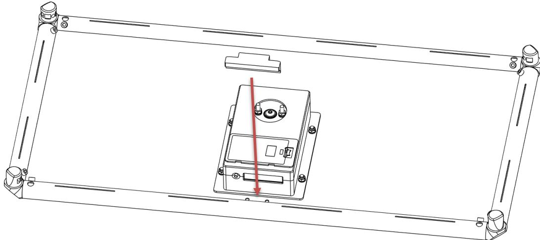
Insert **two buttonhead bolts, 14 mm length**, from the back of the aluminum sheet and tighten securely.
