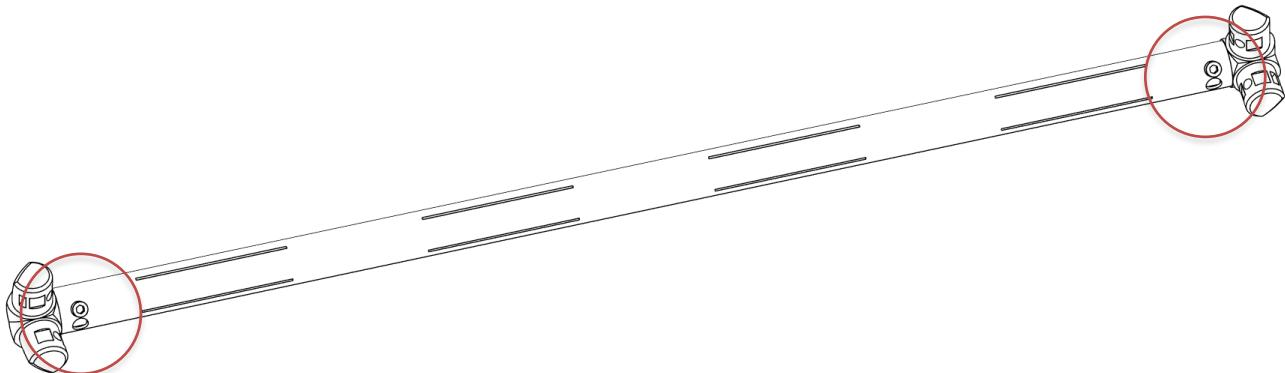
Take one **long tube** (30 mm diameter, 921 mm length). Place the tube so:
