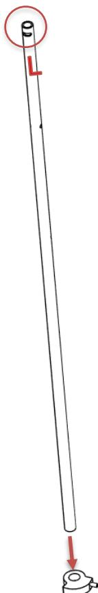
Slide the camblock upward until it reaches the **top marked hole**. Align the set screw with the marked hole in the stainless steel tube.
