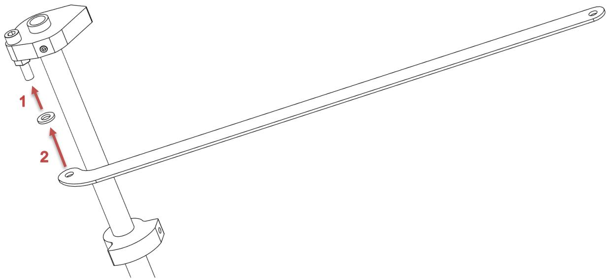
Place a second washer on the bolt. Thread on a **lock nut** (with blue nylon insert). Tighten the lock nut until resistance is felt, then loosen it approximately **1/16 turn**. The linking plate must rotate freely with minimal axial play.
