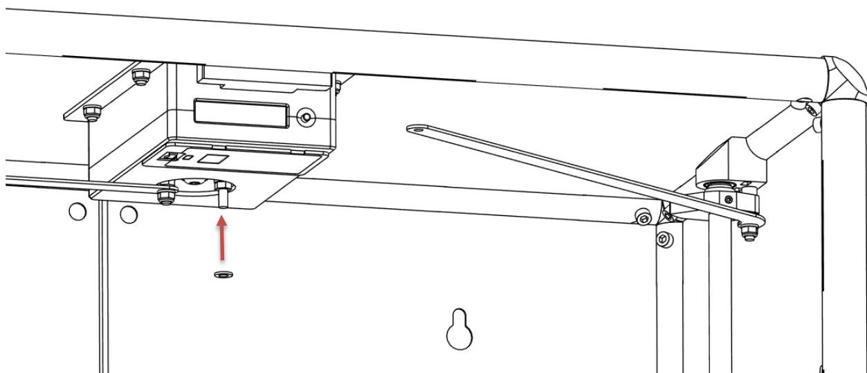
Pull the linking plate slightly downward and place it over the right bolt of the controller. Add a second washer and thread on a **lock nut** (with blue nylon insert).
