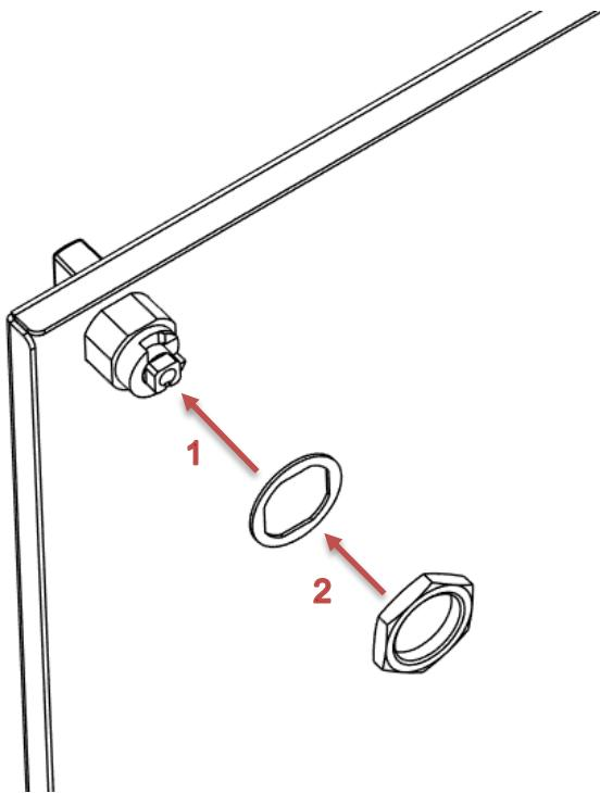
Make sure the knob is pointing downwards and position the lock tongue so it points **upwards**. Insert the bolt and tighten securely using a **10 mm ring spanner**.
