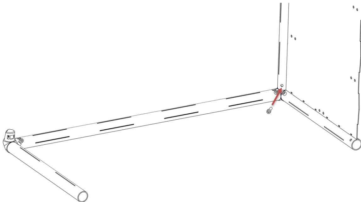
Temporarily secure the end of the long tube to the aluminum sheet using adhesive tape. Repeat this procedure for the **other side panel**.
