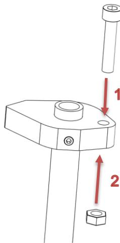
Place a washer onto the Allen bolt. Install the **stainless steel linking plate** using the hole in the **bent end** of the plate. Make sure the linking plate is oriented as shown in the reference image.
