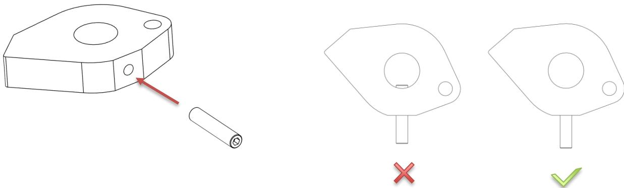
Place the camshaft vertically with the slotted hole at the top. Slide the drive block onto the camshaft. Move the drive block down slightly until the set screw aligns with the **slotted hole** in the tube. Thread in the set screw.
