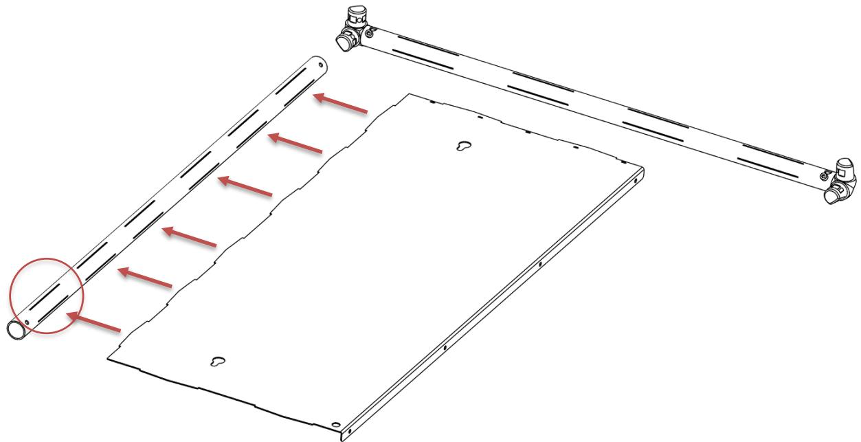
Now slide the long tube and aluminum sheet over the horizontal stub of the left corner piece. At the same time, guide the tongues of the aluminum sheet into the slits of the medium-length tube.
