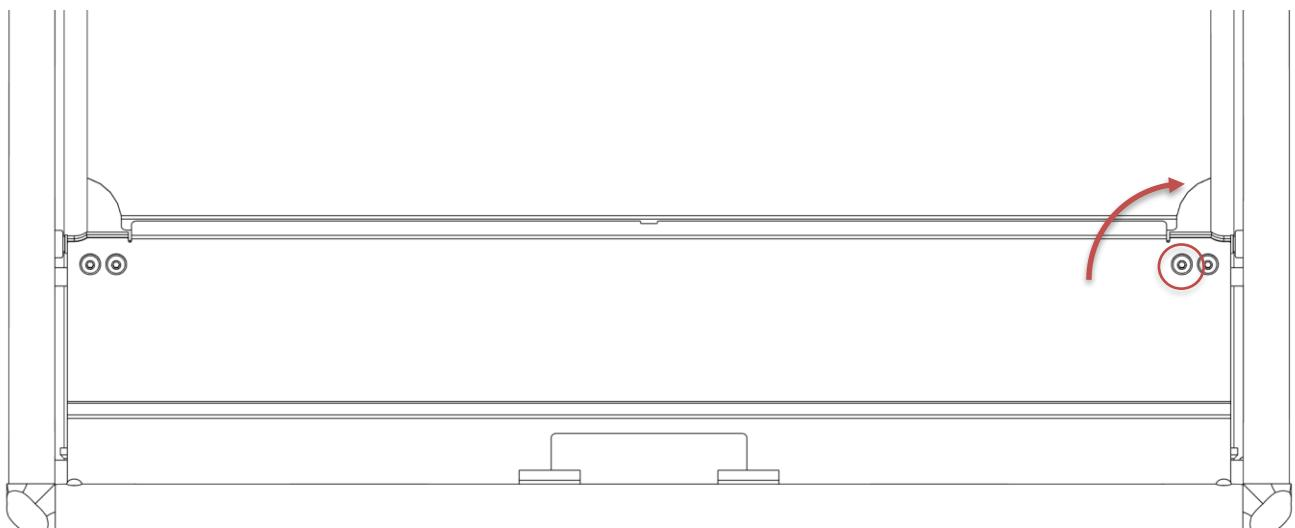
If the second nut was removed earlier, reinsert it now. Hold the nut in place with one finger and insert a **buttonhead bolt, 14 mm length**, through the trapdoor into the hinge. Thread in the bolt and tighten securely using an Allen key.
