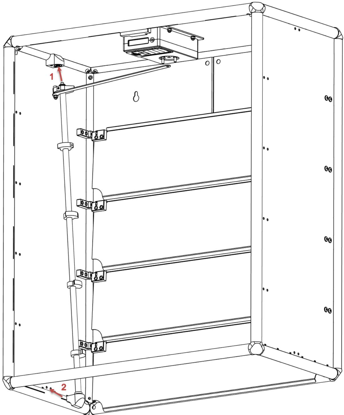
Secure the lower bearing block using **two buttonhead bolts, 14 mm length**.
