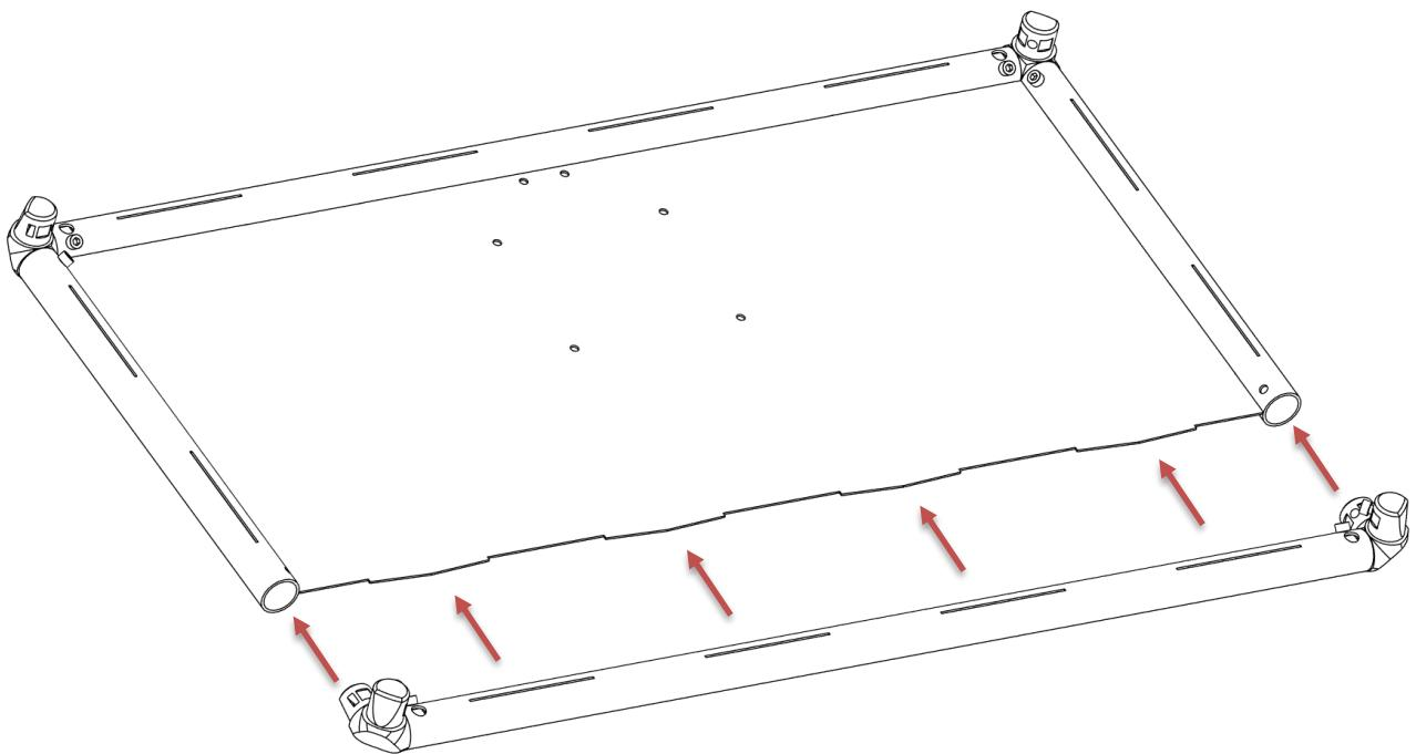
Insert an **Allen bolt, 20 mm length**, through the tube into each corner piece and thread them in lightly.
