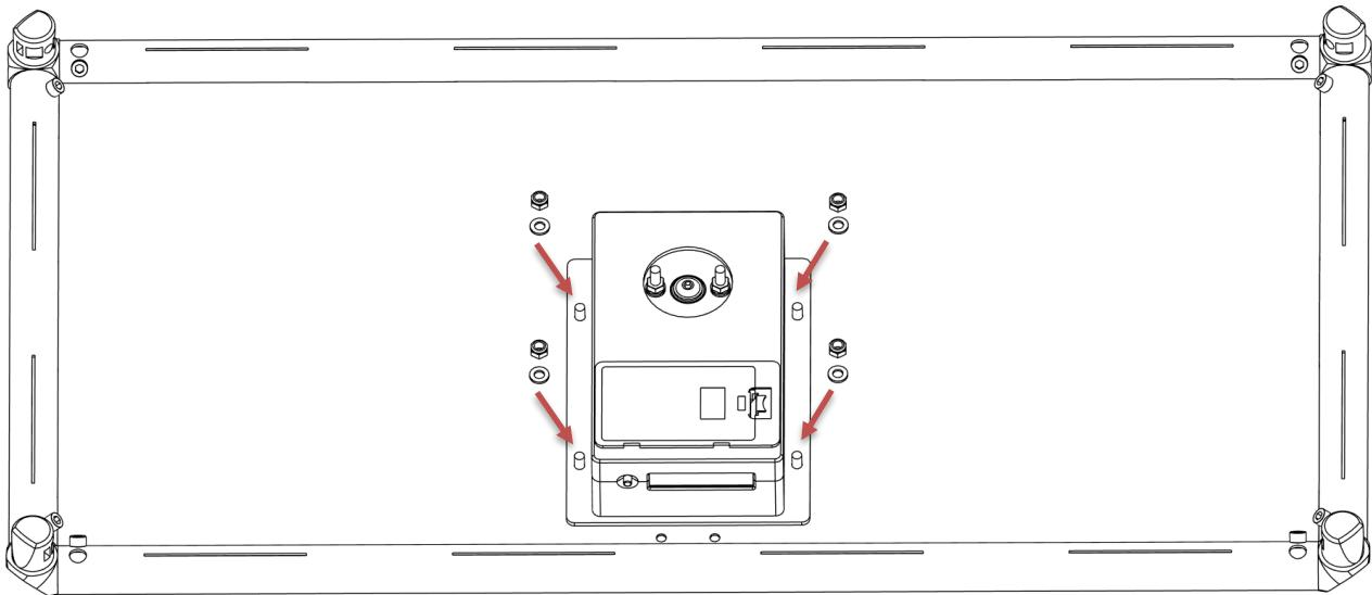
Take the plastic door stop. Insert **two nuts** into the door stop in the same manner as with the corner pieces. Press the nuts in until the holes align.
