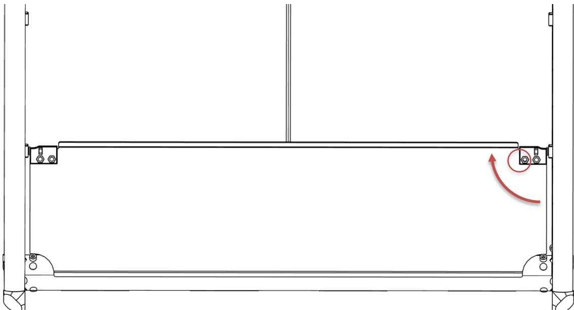
Rotate the trapdoor upward until it is horizontal. If the second nut was removed earlier, reinsert it now. Hold the nut in place with one finger and insert a **buttonhead bolt, 14 mm length**, through the trapdoor into the hinge. Thread in the bolt and tighten securely.
