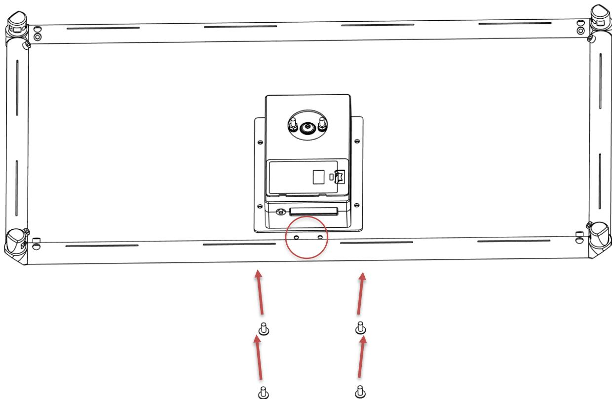
**ATTENTION:** Make sure the controller display faces **towards you** and the display is positioned near the **two holes closest to the front tube**.
