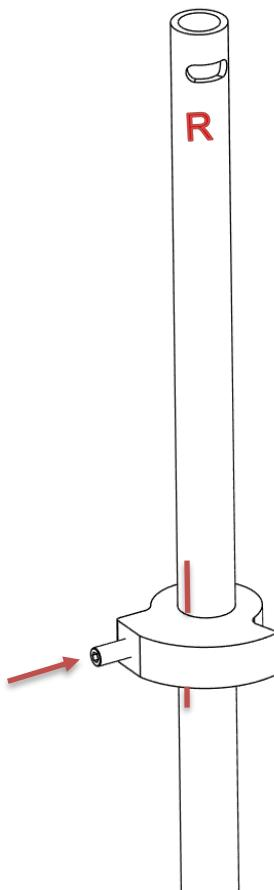
Thread the set screw inward. If resistance is felt before the set screw is fully seated:
