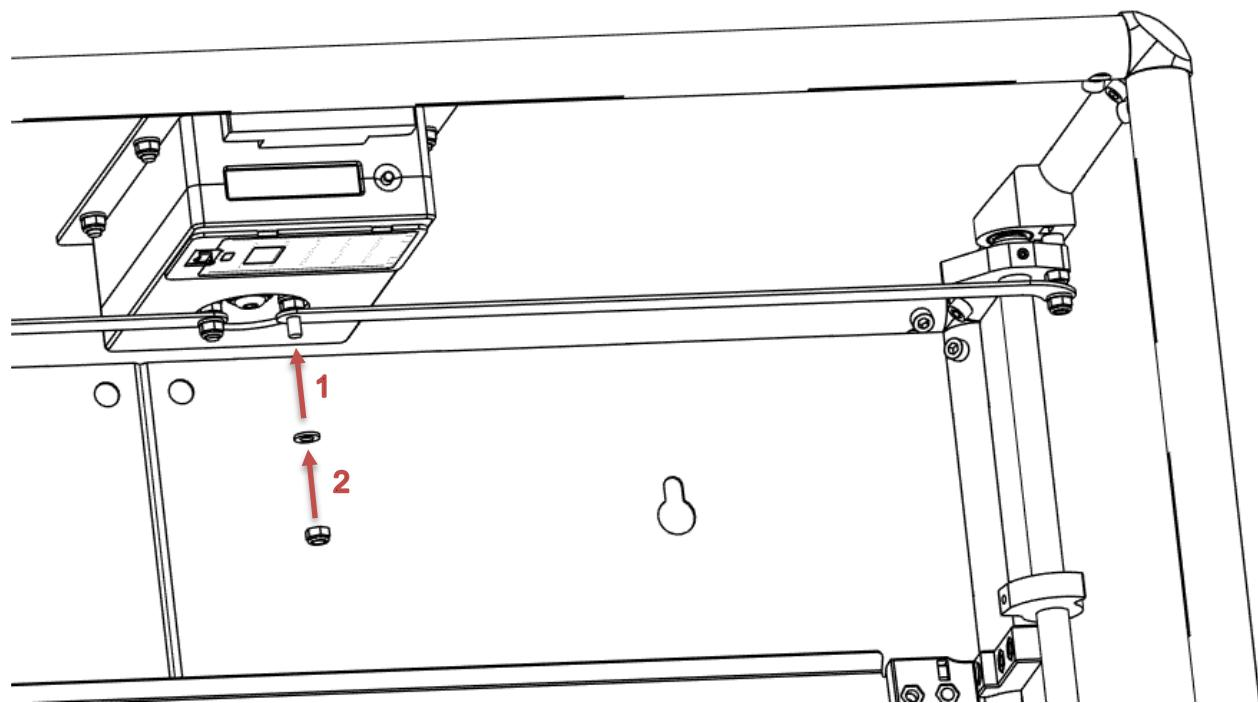
Tighten until resistance is felt, then loosen approximately **1/16 turn** so it can rotate freely without much play between the washers.
