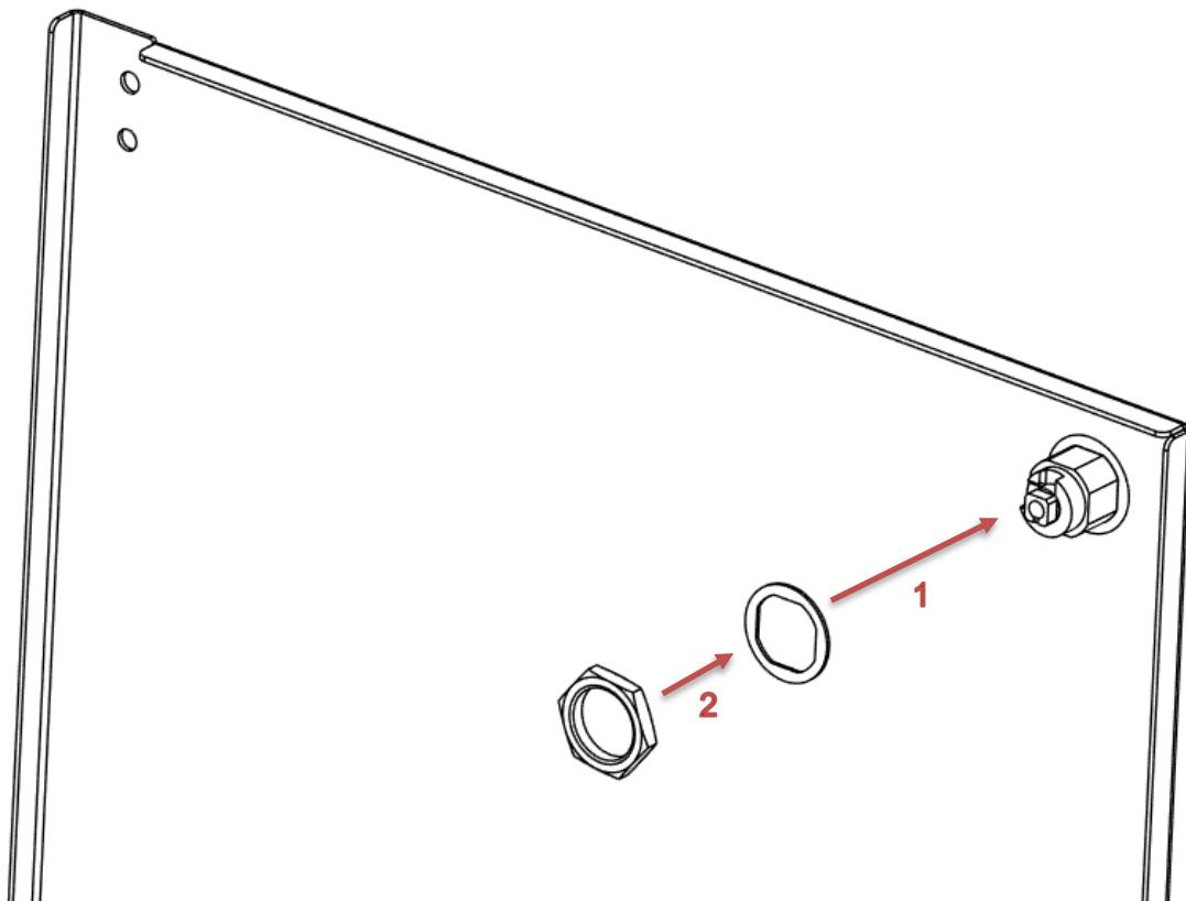
Make sure the knob is pointing downwards and position the lock tongue **upwards**. Insert the bolt and tighten securely using a **10 mm ring spanner**.
