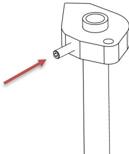
Position the drive block so that the set screw is located **approximately in the center of the slotted hole**. This is the neutral position and will work correctly in most cases. Thread in the set screw until it almost clamps the drive block onto the camshaft. The camshaft must be able to rotate with light hand force. Final tightening will be performed during the camshaft fine adjustment in the last chapter.
