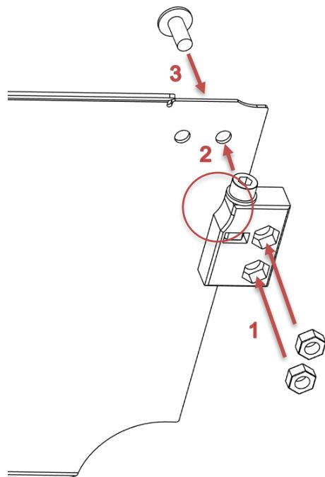
The assembled trapdoor should match the reference image. Repeat this procedure for the **remaining three back trapdoors**.
