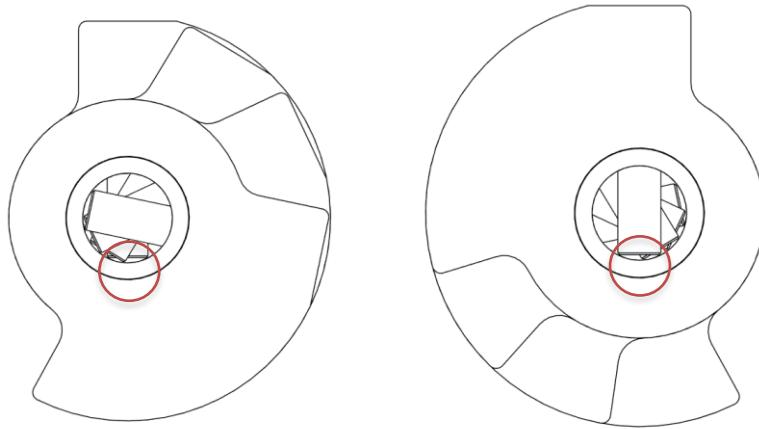
**ATTENTION:** Triple-check this orientation. If the camblocks are installed incorrectly, the trapdoors will not operate correctly and the camshaft must be rebuilt.
