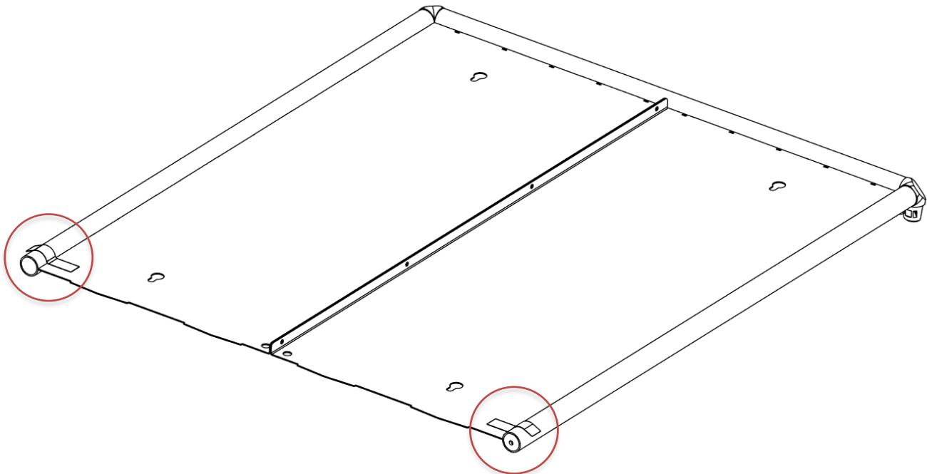
Insert **four buttonhead bolts, 14 mm length**, through the holes in the short flanges of the back panels. Add a washer and nut to each bolt. Align the edges of both flanges accurately.
