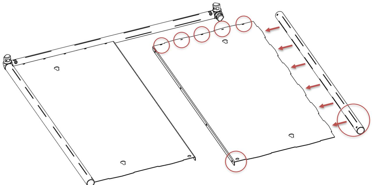
Press both back panel sheets together so the small flanges meet. Slide the tube and sheet over the horizontal stub of the right corner piece. Guide the tongues of the sheet into the slits of the medium-length tube.
