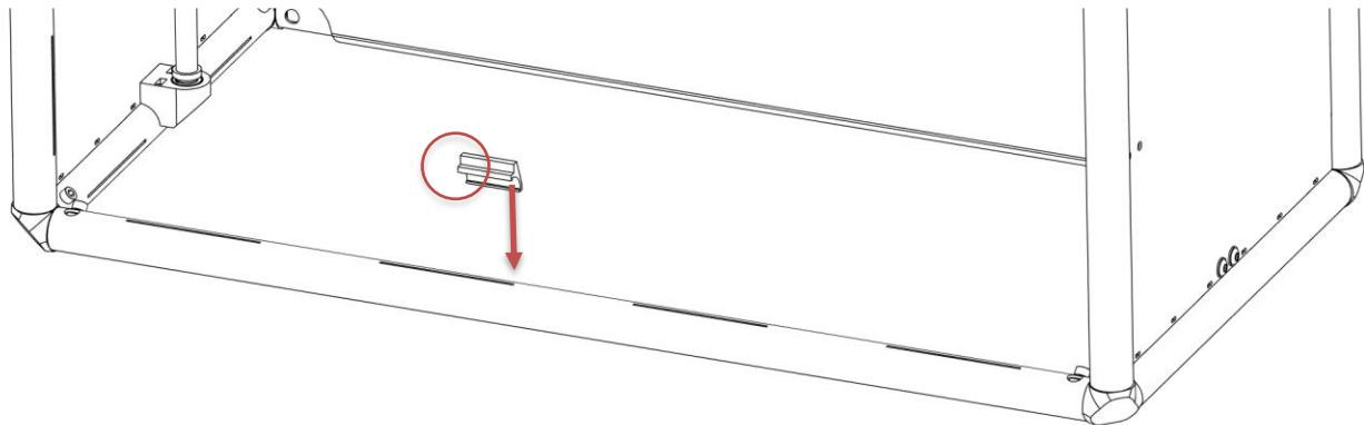
Place the palm of your hand on the door stop and press it **firmly downward** until the **lower ridge snaps into place**.
