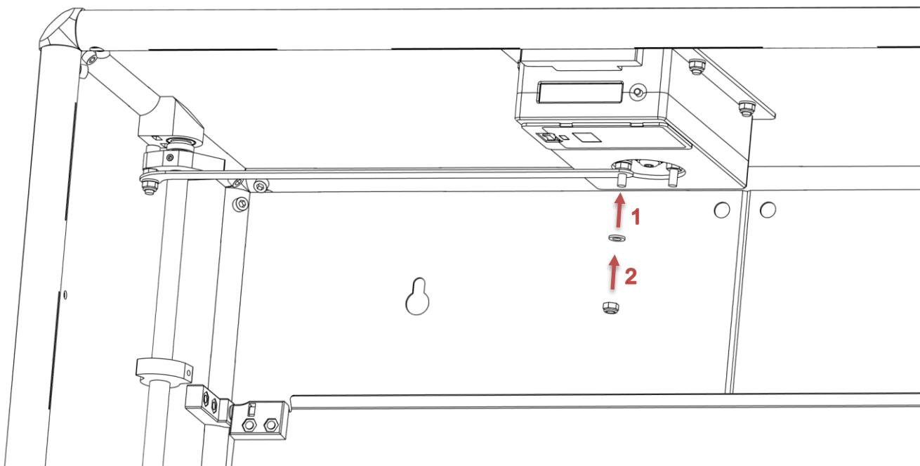
Tighten until resistance is felt, then loosen approximately **1/16 turn** so it can rotate freely without much play between the washers.
