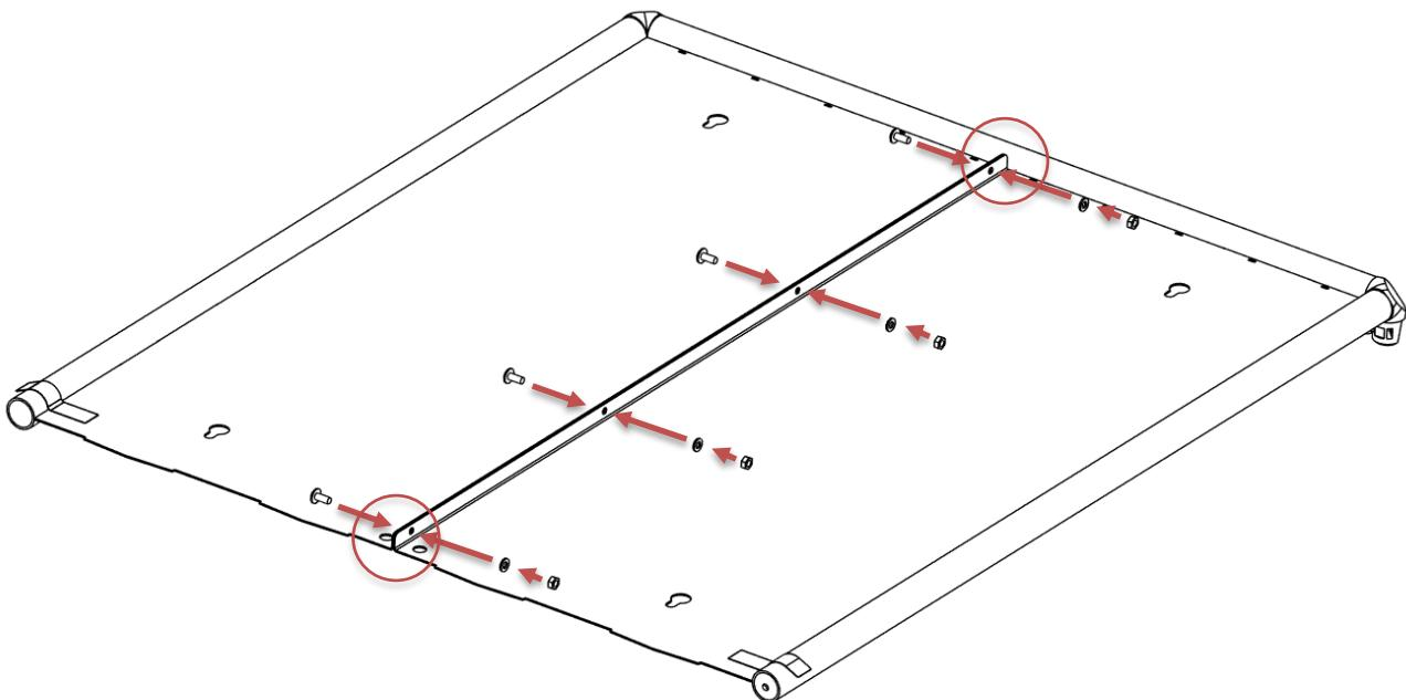
**ATTENTION:** The flanges must be aligned accurately, with no overlap horizontally or vertically.
