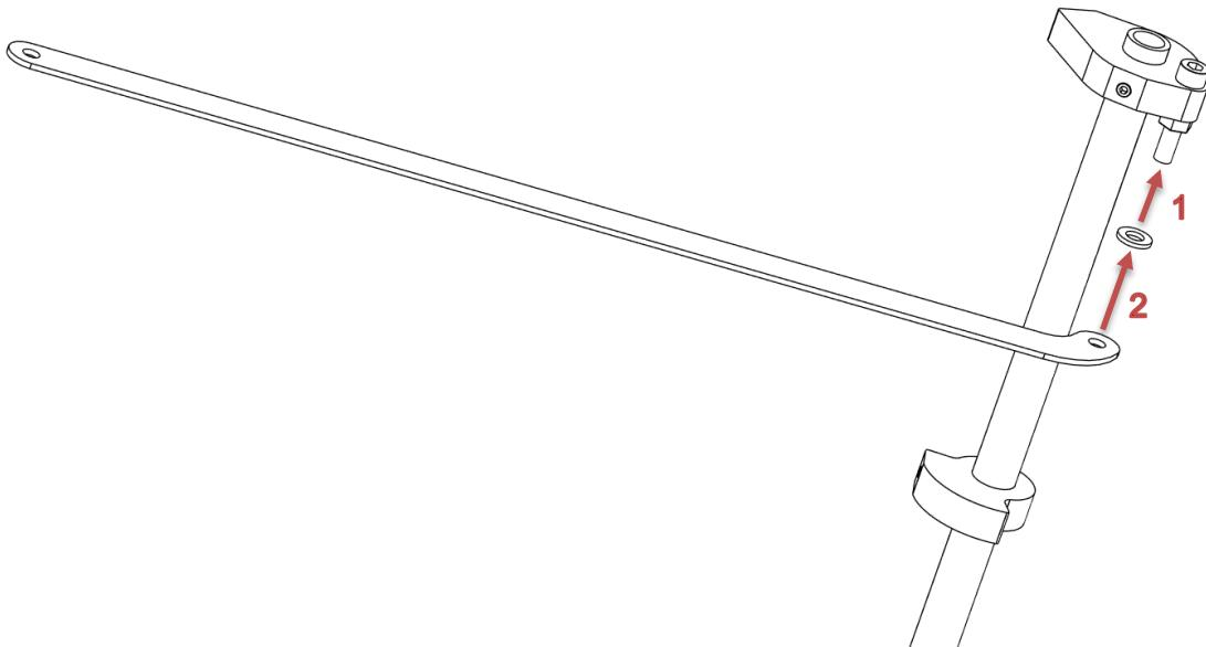
Place a second washer on the bolt. Thread on a **lock nut** (with blue nylon insert). Tighten the lock nut until resistance is felt, then loosen it approximately **1/16 turn**. The linking plate must be able to rotate freely, with minimal axial play between the washers.
