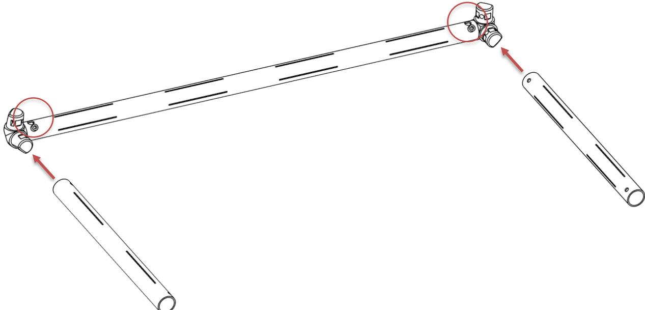
**ATTENTION:** Double-check the orientation of the large hole. This hole will later be used for the door hinge.
