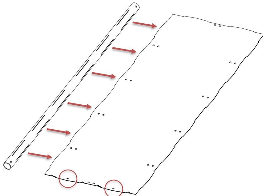
Slide the tube and sheet over the vertical stub of the right corner piece. Guide the tongues of the sheet into the slits of the short tube.
