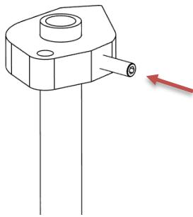
Position the drive block so that the set screw is located **approximately in the center of the slotted hole**. This is the neutral position and will work correctly in most cases. Thread in the set screw until it almost clamps the drive block onto the camshaft. The camshaft must be able to rotate with light hand force. Final tightening will be performed during the camshaft fine adjustment in the last chapter.
