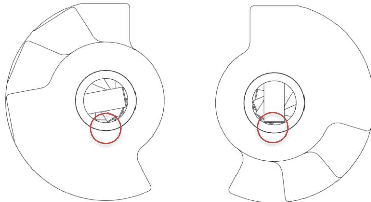
**ATTENTION:** Triple-check the orientation from both top and bottom. If the camblocks are installed incorrectly, the trapdoors will not open in the correct order and the camshaft must be disassembled and rebuilt.
