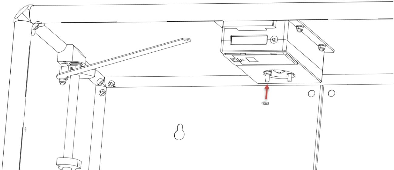
Pull the linking plate slightly downward and place it over the left bolt of the controller. Add a second washer and thread on a **lock nut** (with blue nylon insert).
