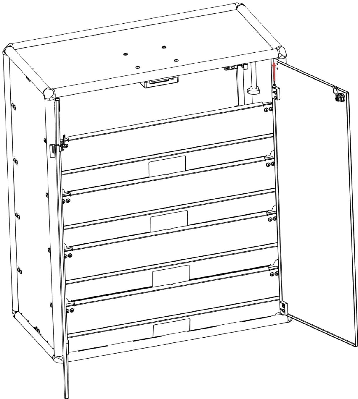
Hold the hinge in place, keeping pressure on the nuts. Insert both buttonhead bolts. Thread them in and tighten securely using an Allen key.
