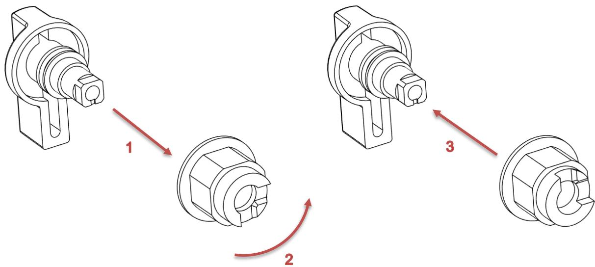
Insert the knob and lock body into the octagonal hole.
