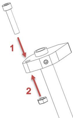
Place a washer on the Allen bolt. Install the **stainless steel linking plate** onto the bolt using the hole in the **bent end** of the plate. Make sure it matches the reference orientation.
