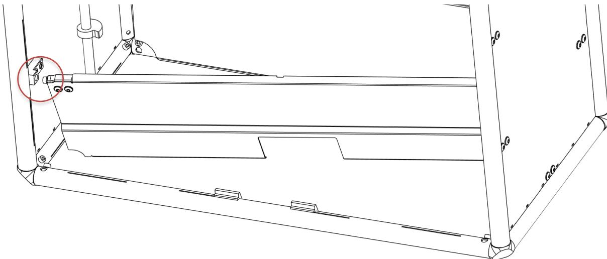
Move the right side of the trapdoor close to the right cabinet hinge. Rotate the trapdoor hinge **clockwise** until it locks into the cabinet hinge and the hole behind the unused nut aligns with the hole in the trapdoor.
