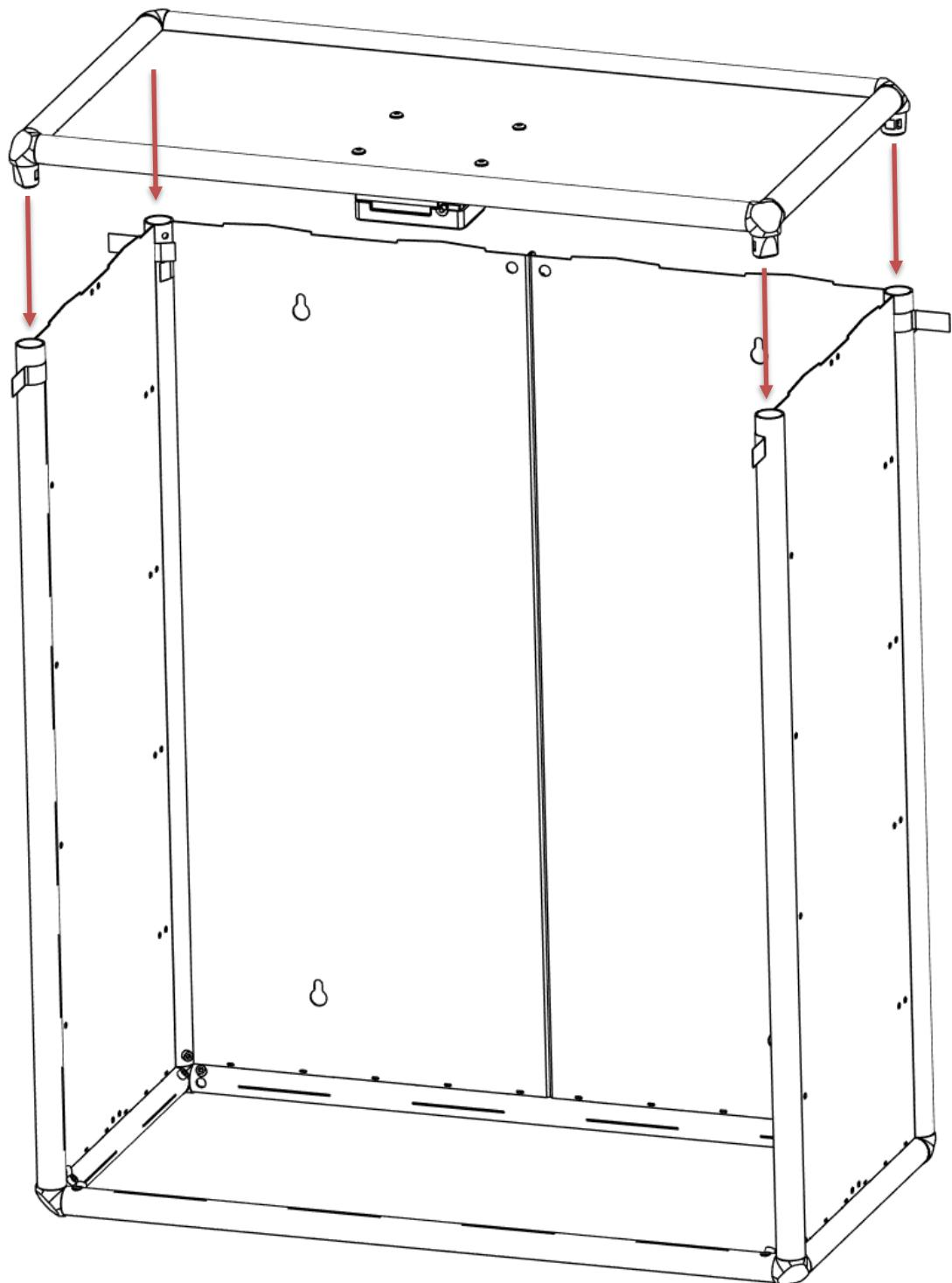
Insert four Allen bolts, 20 mm length, and thread them in lightly. Remove all adhesive tape.
