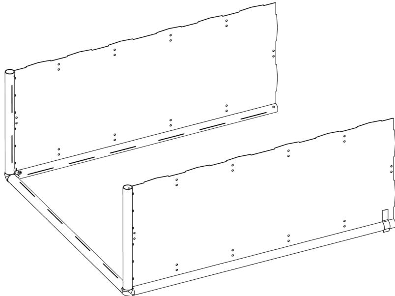
Pick up the back panel assembly. Lower it carefully onto the side panel assembly:
