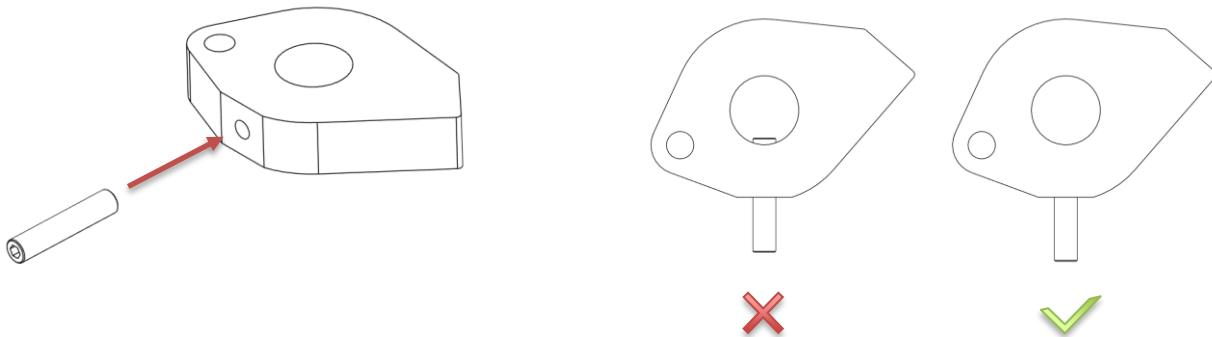
Place the camshaft vertically with the slotted hole at the top. Slide the drive block onto the camshaft, aligning the set screw with the slotted hole. Thread in the set screw.
