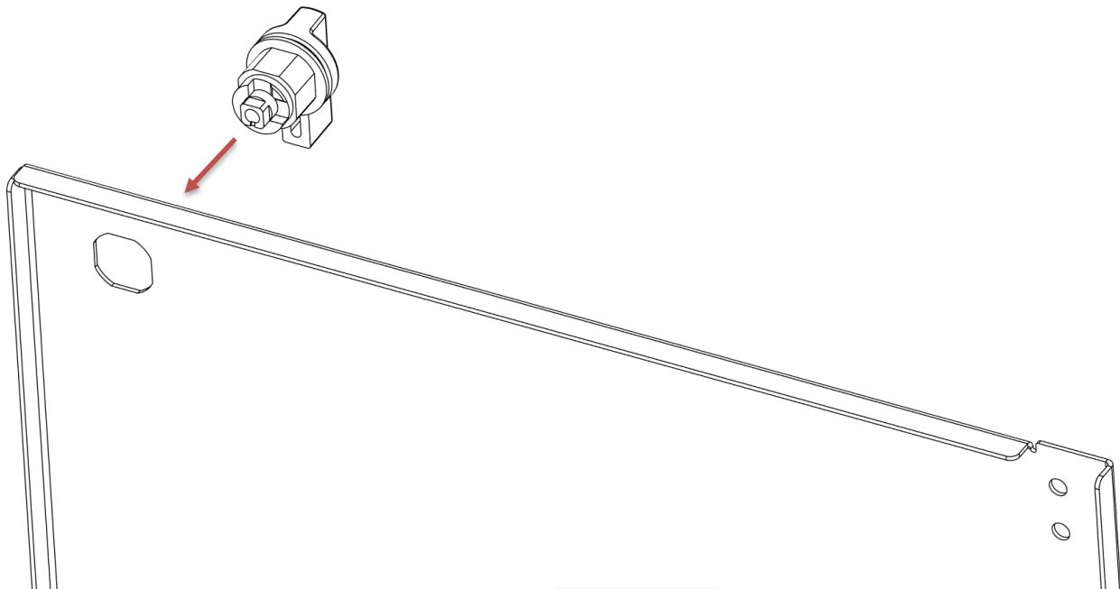
**ATTENTION:** Make sure the knob points **downwards** and the two slots in the lock body are oriented exactly as shown in the reference image.
