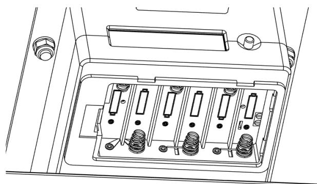
When the last battery is inserted, the HayTimer will automatically power up and the display will switch on.
