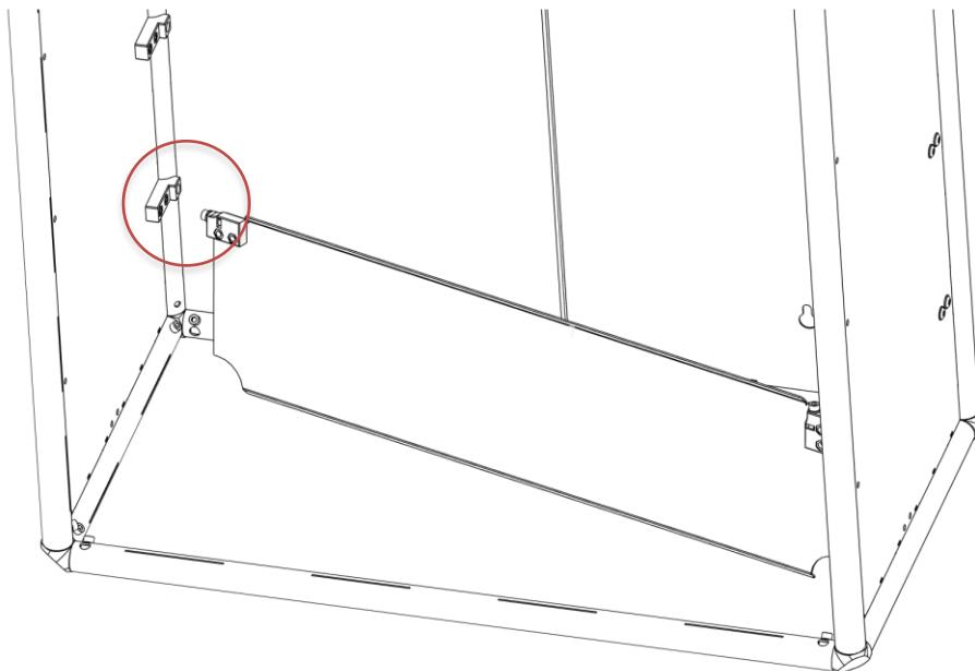
Move the right side of the trapdoor close to the right cabinet hinge. Rotate the trapdoor hinge **clockwise** until it locks into the cabinet hinge and the hole behind the unused nut aligns with the hole in the trapdoor.
