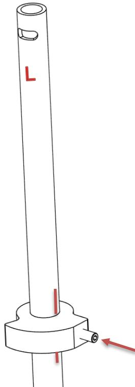
Thread the set screw inward. If resistance is felt before the set screw is fully seated:
