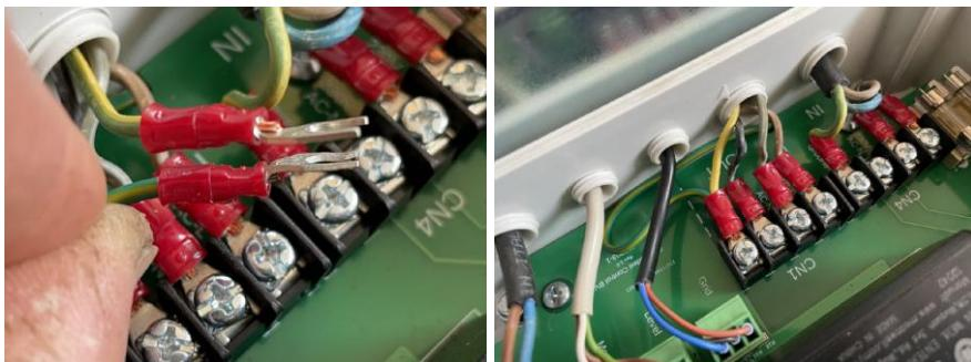
Pull the wires up a little while sliding the sync cable into the swivel. Slide this until about 5 mm of the black jacket comes out of the swivel. Then tighten the swivel firmly by hand. Check whether the synchronization cable is secure by pulling it out of the controller unit, it must not slide out of the swivel.
