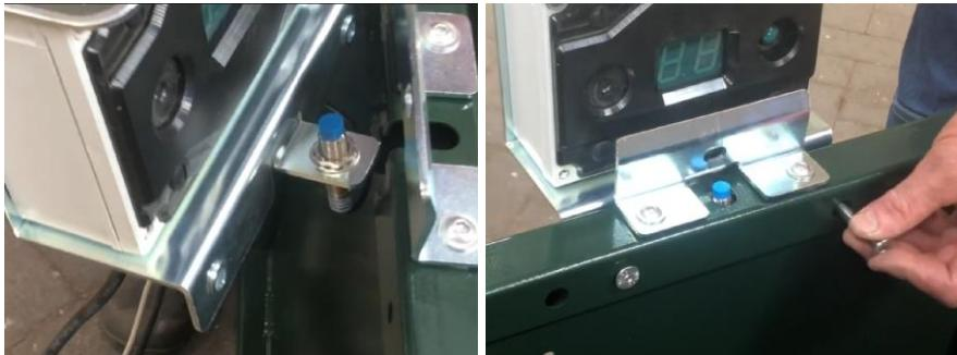
Place a mounting bracket against the back of the FeedingMaster. Secure this first with a countersunk M8x60 bolt, tighten it by hand as far as possible. Then place an M8x20 flange bolt in the hole just above the feeding base, tighten it by hand as far as possible.
