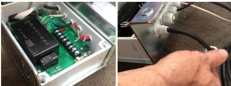
Place the synchronization cable by inserting all four fork cable lugs one after the other through the gland. Both sides of the synchronization cable are equal, so it does not matter which side is used.
