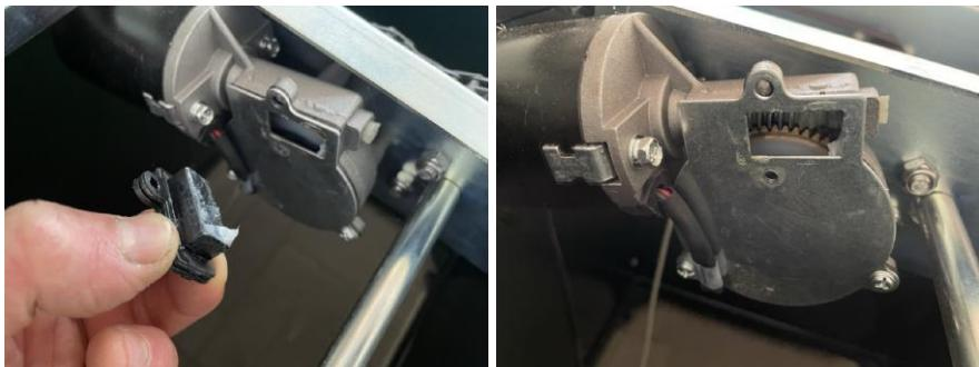
Place the black cap back in the motor and secure it with the two screws, the longest screw goes into the top hole. Spray some White Grease between the axles and the black bearing blocks. Rotate the turning shafts a few times to spread the grease.
