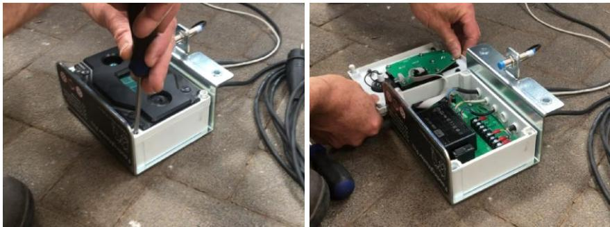
In addition to the gland through which the power cord is fed, a second gland is present for the synchronization cable. It is fitted with an M6 flange bolt to seal it, unscrew the swivel and remove the flange bolt.
