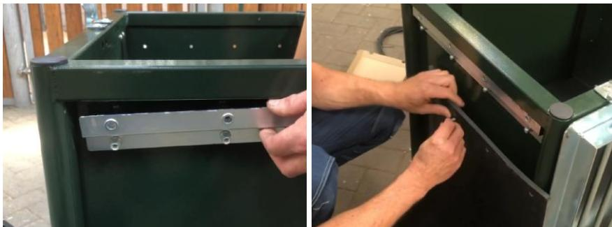
Place it in front of the appropriate hole in the suspension bracket and screw it on by hand. Push the remaining four M8x25 flange bolts through the holes in the rubber plate and tighten them by hand. Retighten the flange bolts by half a turn.
