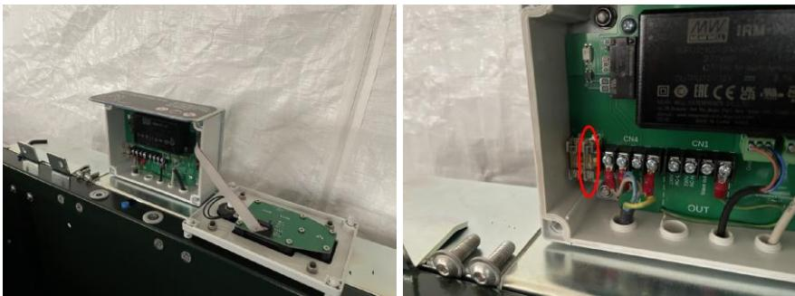
Place the front panel in front of the controller. Push the display cable towards the lower right corner of the housing. Place the front panel on the controller. Check whether it is flush with the housing on all sides. The front panel must touch the housing without resistance, never press it if this is not the case. In that case, check that there are no wires between the front panel and the controller.
