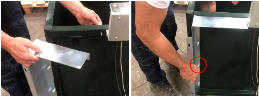
Install the second M8x60 countersunk bolt and the second M8x20 flange bolt. Repeat for the other mounting bracket. Fold the feeding base forward and place the M8x20 flange bolts in the bottom holes of the mounting brackets. Tighten these by hand as far as possible and tighten with the Allen key.
