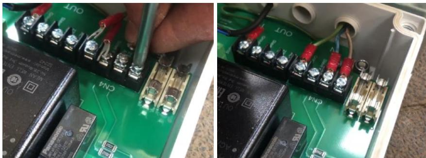
Pull the wires up a little while the power cord is being pushed into the swivel. Slide this until about 5 mm of the black jacket comes out of the swivel. Then tighten the swivel firmly by hand. Check whether the power cord is firmly attached by pulling it out of the controller, it must not slide out of the swivel.
