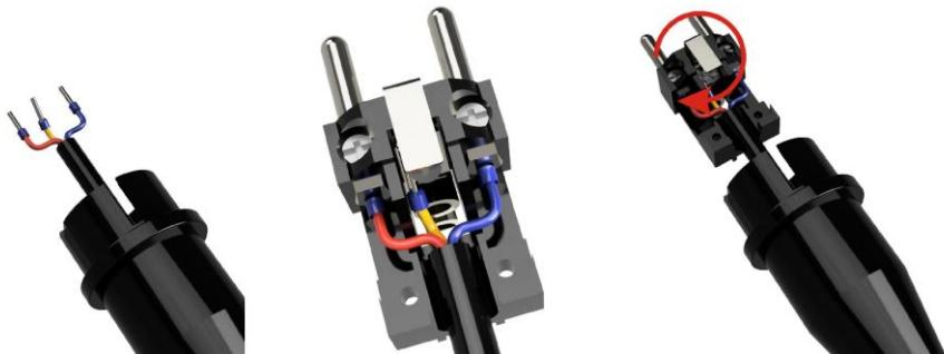
Place the red strain relief over the outer sheath of the power cable, the convex side must point away from the power cable. Place and tighten the two screws of the strain relief so that the power cable can slide. Push the power cable towards the contacts of the power plug. The outer casing must be visible at least 2 mm behind the strain relief. Tighten the two screws of the strain relief firmly, when the power cable is pulled, no movement of the wires should be visible.
