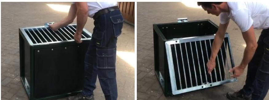
Remove the mounting brackets and box of installation material from the FeedingMaster. Tilt the grid slightly away from the rubber protective flap, then tilt the FeedingMaster forward so that it remains at an angle. Lift the controller with the power cord in one hand and tilt the feeding base forward with the other hand.
