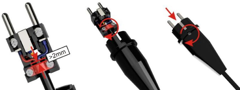
There is a hole in the middle grounding plate at the front of the power plug. Rotate the housing of the power plug so that the locking screw in the housing is at this hole, then slide the power plug into the housing. Then tighten the locking screw.
