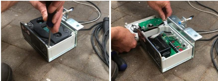
Unscrew the swivel from the strain relief through which the power cord is fed. Unscrew the three connections of the connector on the controller marked CN4 (In) two turns. Remove the spade cable lugs by sliding them out from under the terminals. Remove the power cord by pulling all three forked cable lugs out of the swivel one after the other.
