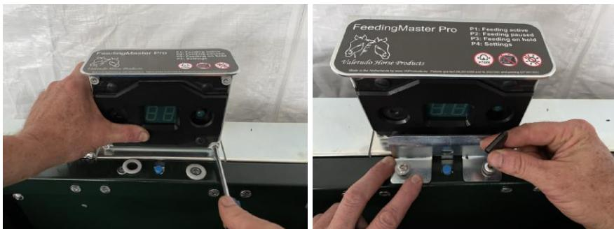
Tilt the grid back up and let it fall gently over the strike plate until you hear a clear 'click' from the locking pin. Slide the strike plate parallel to the grid at approximately 1 mm from the grid. Tighten the two M8x20 flange bolts securely. Check the correct operation of the locking pin.
