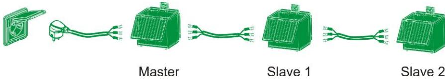
**WARNING:** Never connect more than 4 Slave FeedingMasters to a Master. The Master is then overloaded with the risk of fire hazard.
