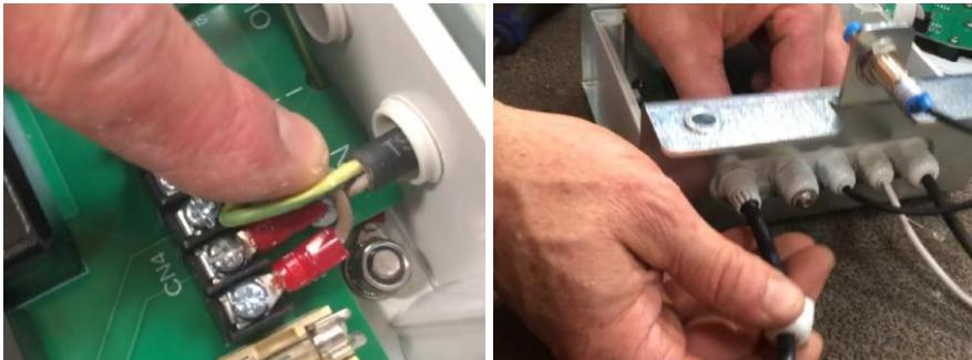
Place the front panel in front of the controller. Press the display cable towards the bottom right corner of the housing. Place the front panel on the controller. Check whether it is flush with the housing on all sides. The front panel must touch the housing without resistance, never press it if this is not the case. In that case, check that there are no cables between the front panel and the controller.
