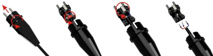
Unscrew and remove the two screws from the strain relief. Loosen the three screws that secure the connecting wires to the power plug by one turn. The power cord can be removed.
