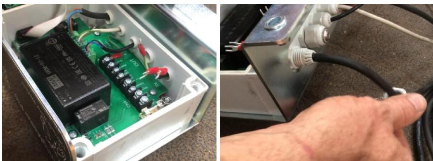
Remove the power cord by pulling all three forked cable lugs out of the swivel one after the other. Install the 10 meters power cord by inserting all three forked cable lugs one after the other through the swivel. Slide the fork cable lugs into the terminals of the connector on the controller marked CN4 (In). The third connection marked "Slave" In is not used. Connect the wires as follows:
