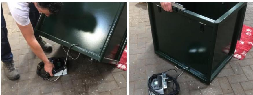
When the cables between the FeedingMaster and the controller are twisted together, turn the controller over until the cables hang neatly next to each other.
