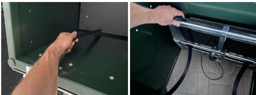
**WARNING:** Tilt the feeding base **never** from back to front. This can cause the drive unit cables to get caught in the drive unit and cause permanent damage.
