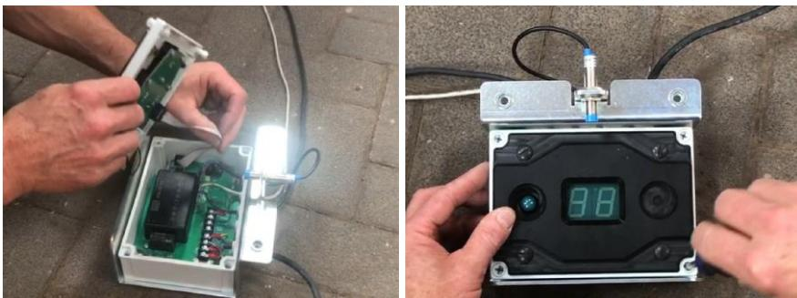
**WARNING:** Never place the front panel on the controller at an angle. The controller is no longer waterproof, which can lead to malfunctions and damage.
