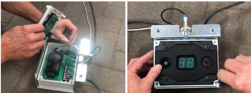
Tighten the four gray screws on the corners of the controller housing by hand. Then turn them clockwise 1/8 turn.
