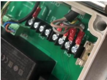
On the Slave, another FeedingMaster can be connected using a synchronization cable to the connections of the connector on the controller which is marked with CN1 (Out). In that case, follow the instructions as indicated in the chapter 'Connecting to the Master' to connect the synchronization cable to the Slave.
