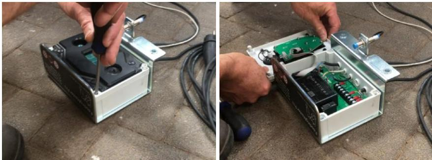
Unscrew the swivel from the strain relief through which the power cord is fed. Unscrew the three connections of the connector on the controller marked CN4 (In) two turns. Remove the spade cable lugs by sliding them out from under the terminals.
