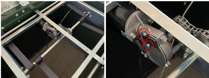
Pull the black cap out of the motor to expose the gears. If there is plenty of grease that has been pressed against the wall of the motor, this can be scraped off the wall with a fine screwdriver and lubricated over and between the teeth of the gears. If no grease is visible, place a teaspoon of White Grease or Vaseline over and between the gears.
