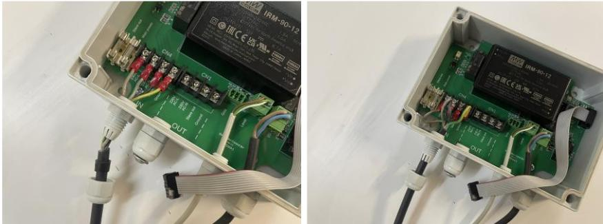
Pull the wires up a bit while sliding the sync cable into the swivel. Slide it just until about 5 mm of the black sheath comes out of the swivel. Then tighten the swivel firmly by hand. Check that the synchronization cable is secure by pulling it out of the controller, it should not slide out of the swivel.
