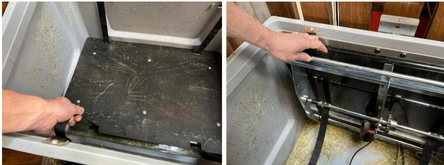
**WARNING:** Never tilt the feeding base from back to front. This can cause the drive cables to get caught in the drive, causing permanent damage.
