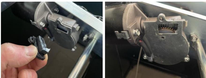
Place the black cap back in the motor and secure it with the two screws, the longest screw goes into the top hole. Spray some White Grease between the axles and the black bearing blocks. Rotate the turning shafts a few times to spread the grease.
