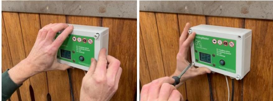
Hand tighten the four gray screws which are at the corners of the control housing. Then tighten them 1/8 turn clockwise.
