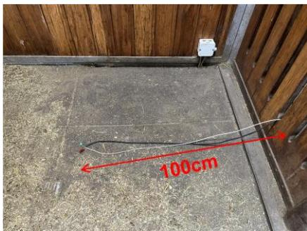
**WARNING:** Do not exceed the maximum distance between the FeedingMaster and the controller. During the movement of the feeding base, the connecting cables are pulled into the FeedingMaster. If they do not have enough space to move, the drive can pull them apart which can lead to permanent damage.
