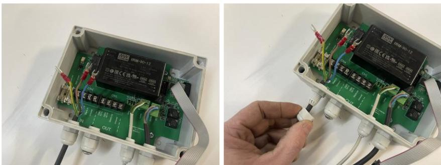
To make passing the synchronization cable easier, the swivel can be unscrewed completely. Slide it over the synchronization cable. You can also remove the black rubber ring from the gland that is still screwed into the housing. Slide the rubber ring over the synchronization cable as well.
