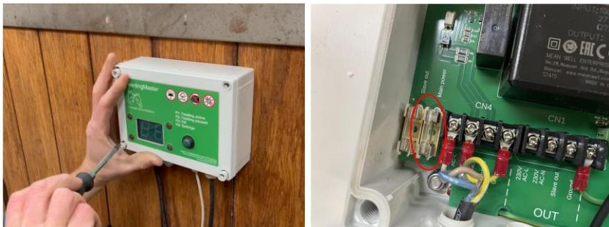
In the lower left corner of the control two fuses are visible. The left fuse is to protect the Slave input, the right fuse is the main fuse of the control. Remove it by flipping the fuse out of the holder. Check if the fuse is defective. If so, replace it with the same type (250 VAC, 1A, slow, 5x20 mm).
