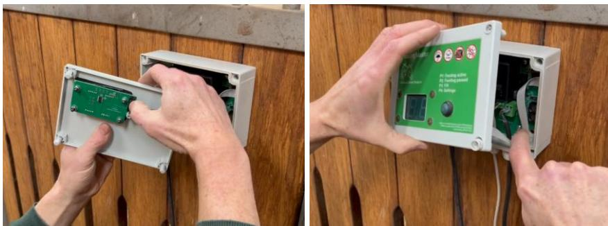
Place the front panel in front of the controller. Push the front panel cable in the direction of the right lower corner of the housing. Place the front panel on the controller. Check that it connects smoothly with the housing on all sides. The front panel should touch the housing without resistance, never press it if it does not. In this case, check that there are no cables between the front panel and the controller.
