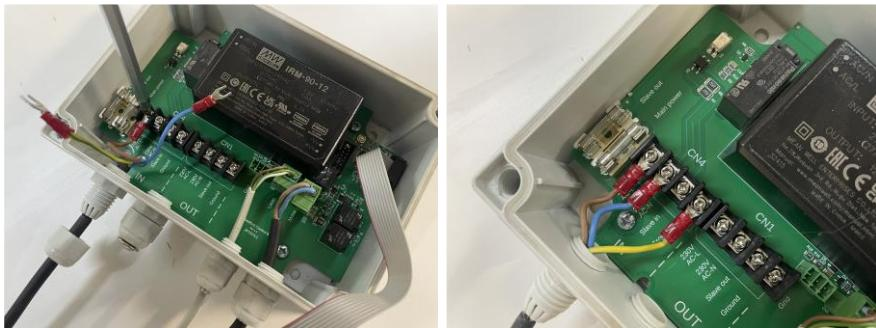
Pull the wires up a bit while sliding the power cord into the swivel. Slide it just until about 5 mm of the black jacket comes out of the swivel. Then tighten the swivel firmly by hand. Check that the power cord is secure by pulling it out of the control, it should not slide out of the gland.
