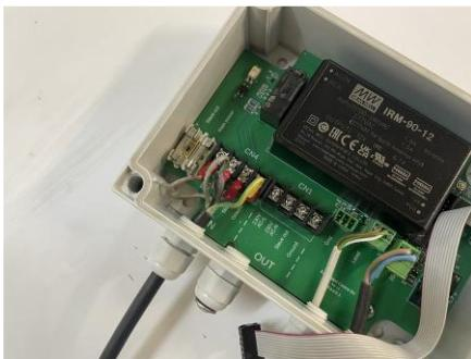
On the Slave, a subsequent FeedingMaster can be synchronized using a synchronization cable connected to the terminals of the connector on the control marked CN1 (Out). In this case, follow the instructions indicated in the “Connecting to the Master” section to connect the synchronization cable to the subsequent FeedingMaster.
