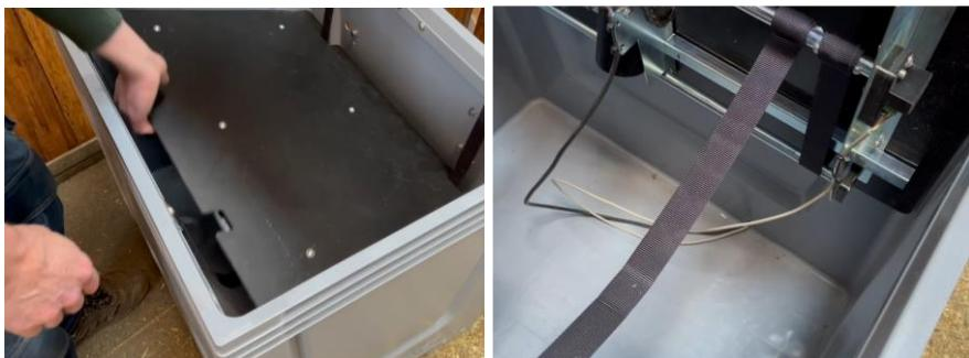
Gently lower the feeding base back into place. Now fold it away from you. Check that both connection cables can move freely and are not stuck between the suspension straps and the drive. Both connection cables must run under the front suspension straps. Gently lower the feeding base back into place.
