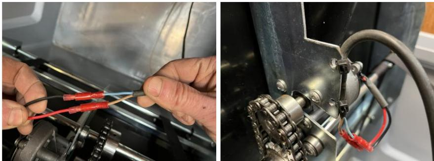
Place the black connection cable against the metal of the feeding base, it should point away from the motor. Insert a cable tie through the hole in the metal of the feeding base and tighten it. Place a second cable tie through the second hole in the metal of the feeding base and tighten it. Cut off the excess parts of both cable ties.
