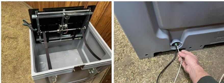
Fold the feeding base toward you so that the holes in the back wall become visible. If necessary, secure it with a clamp so that it stays upright. Insert both connection cables into the FeedingMaster through the hole in the bottom right-hand corner of the back wall.
