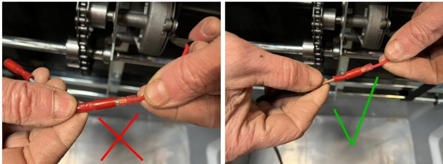
Insert the plug of the black motor wire into the socket of the blue wire. Push it in as far as possible, there should be no metal visible from the plug.
