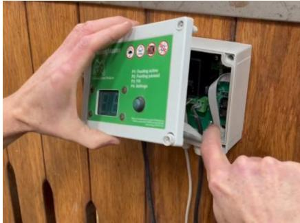
Place the front panel in front of the controller. Push the front panel cable towards the bottom right corner of the housing. Place the front panel on the controller. Check that it fits smoothly with the housing on all sides. The front panel must touch the housing without resistance, never press it if this is not the case. In that case, check that there are no cables between the front panel and the control.
