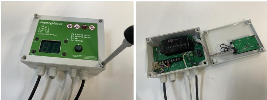
To make it easier to mount the controller, the front panel can be temporarily disconnected from the controller. To do this, carefully pull the black plug out of the front panel.
