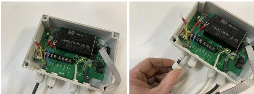
Remove the power cord by pulling all three fork cord lugs out of the swivel one after another.
