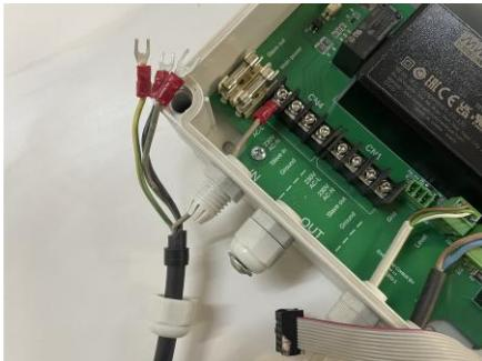
Now feed one wire at a time through the swivel in the controller and connect the fork cable lug to the connector. Both sides of the synchronization cable are the same, so it does not matter which side is used. Then connect the next wire.
