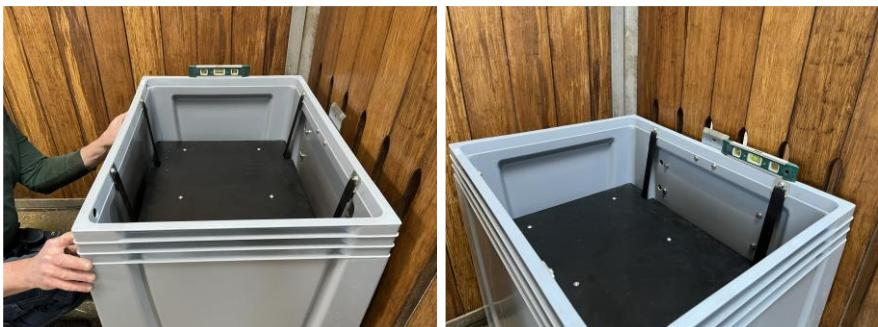
Check that the FeedingMaster is level in both depth and width. To level the FeedingMaster, adjustment plates can be placed under the legs of the FeedingMaster provided they are no more than 5 mm thick.
