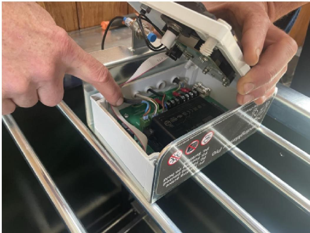
[ ] Place the front of the housing on the controller housing. Check that there are no wires between the parts and that the front of the housing rests neatly on the back of the housing.
