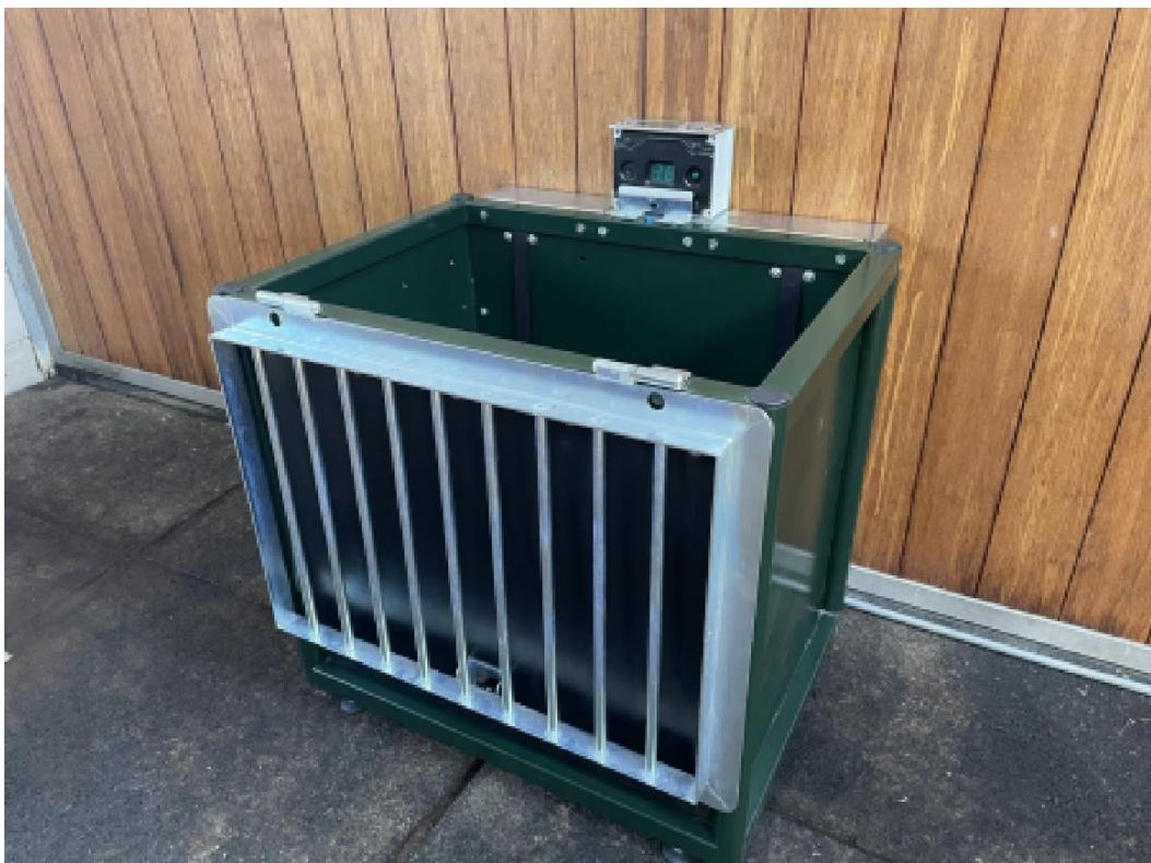
[ ] Remove the two allen screws holding the controller using a 5mm allen key.
