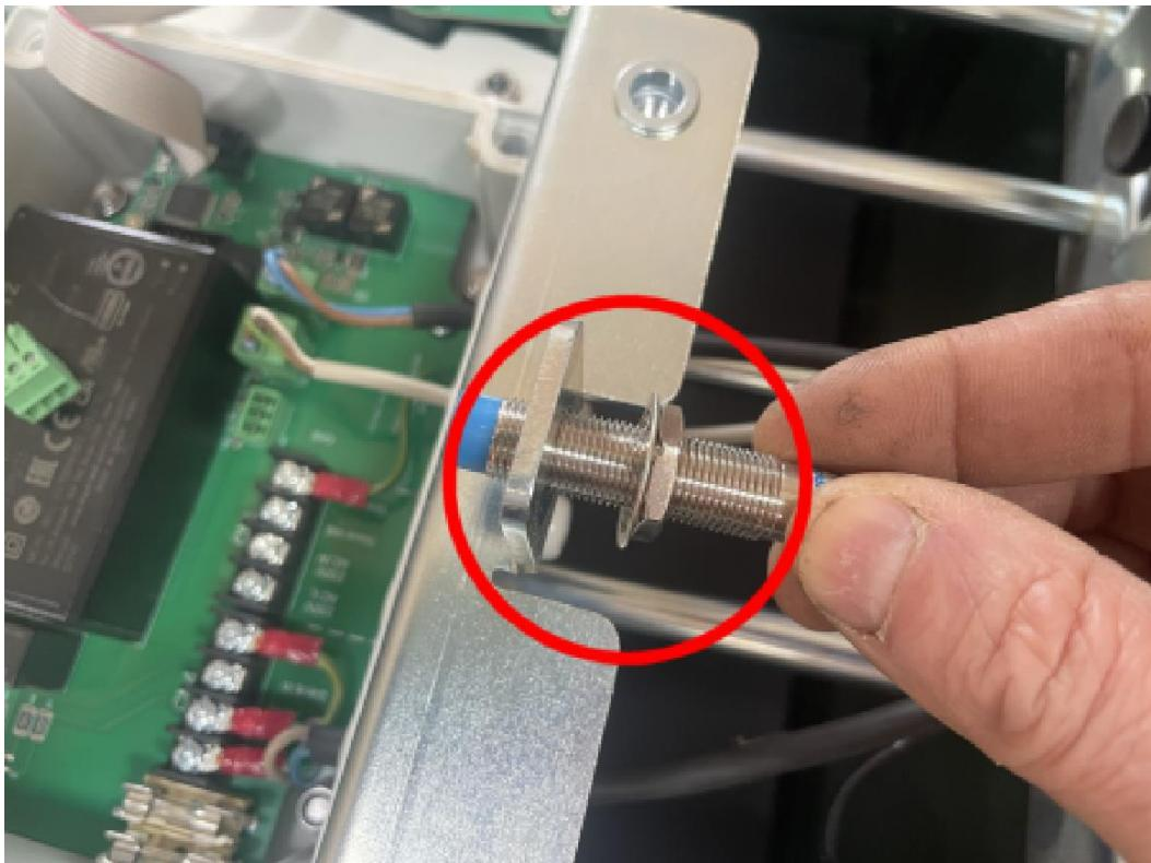
[ ] Place a knurled ring on the other side over the sensor against the controller. Place the second nut on the sensor and hand tighten.
