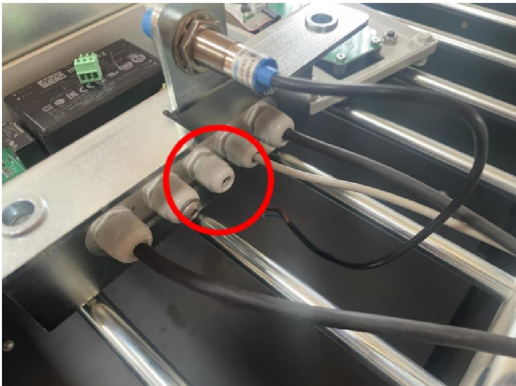
[ ] Place two 17mm spanners on the nuts of the grid sensor and loosen the nuts.
