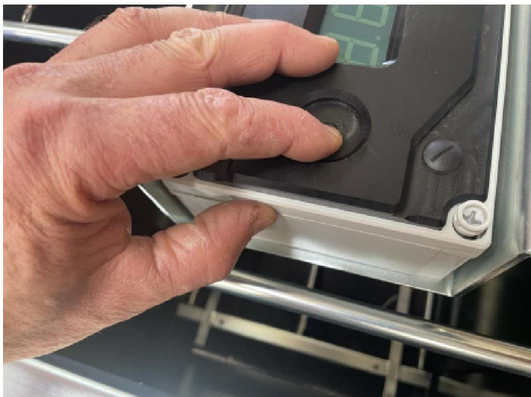
[ ] Secure the front of the housing by finger-tightening the four nuts. Tighten the nuts 1/8 turn of the screwdriver.
