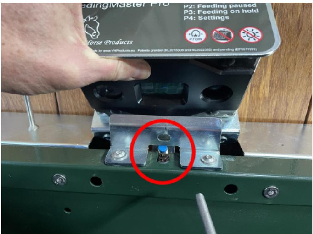
[ ] Tilt the controller back. Secure the controller with two M8x60 countersunk bolts.
