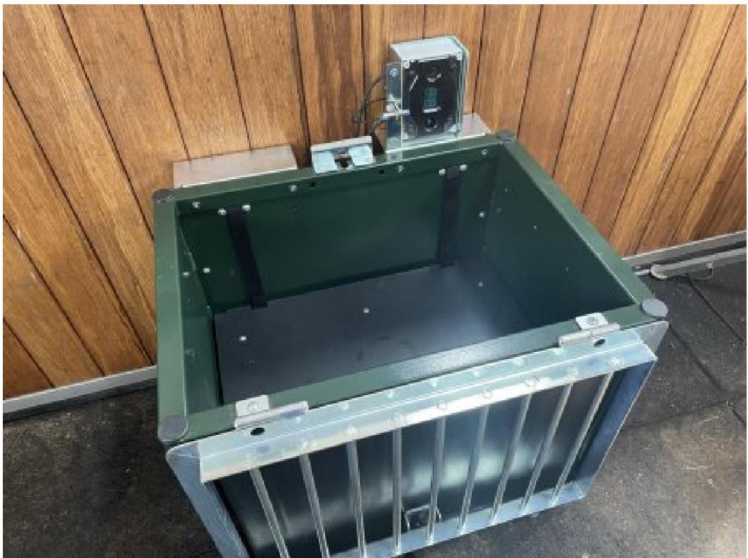
[ ] Grab the controller and tilt it forward. Lower the controller between the mounting brackets. Hook the grid sensor into the recess under the grid closure bracket.
