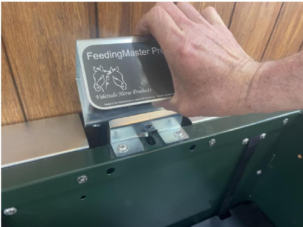
[ ] Lift the controller between the mounting brackets.
