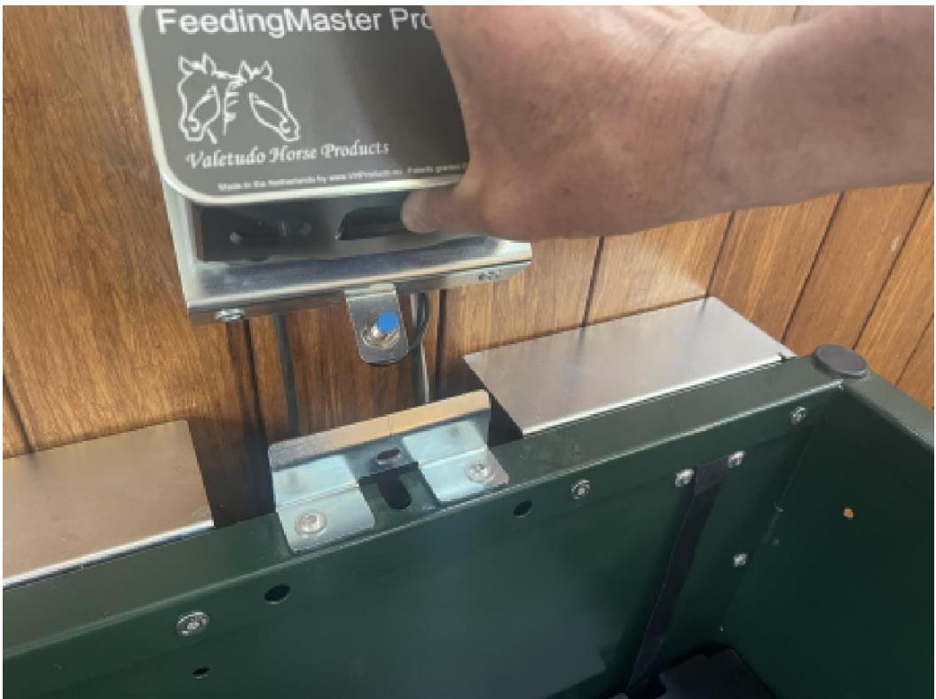
[ ] Tilt the controller 90 degrees clockwise and place it on the right mounting bracket.
