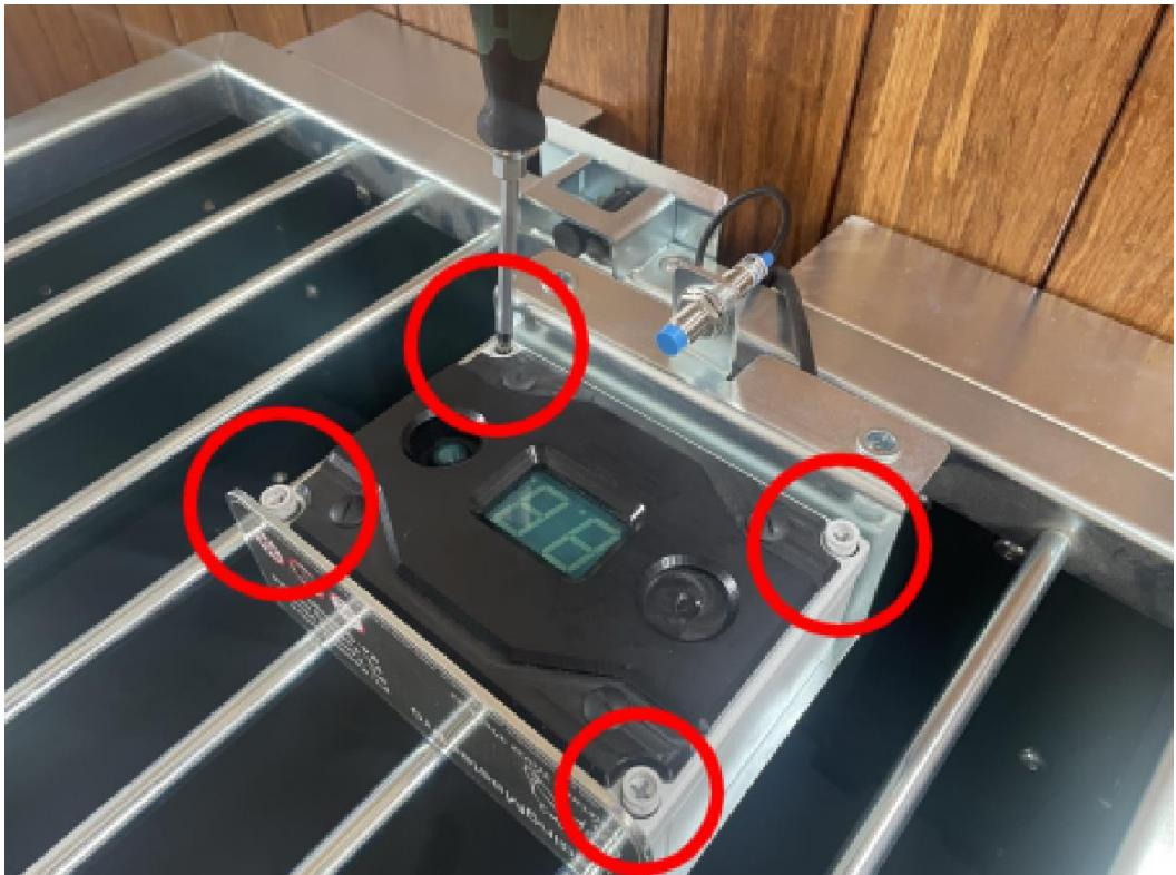
[ ] Lift the front of the housing and place it to the left of the controller.
