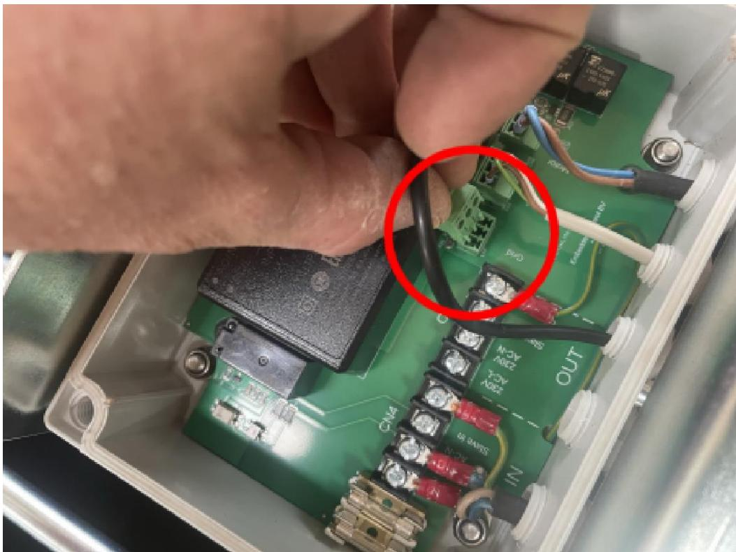
[ ] Gently pull the cable of the grid sensor out of the strain relief until it is as short as possible but not yet under tension.
